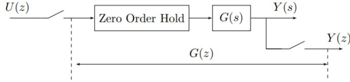
where  $G(s)$  is the transfer function of a continuous-time system and the latches represent sampling. Show that the transfer function from  $U(z)$  to  $Y(z)$  is,
