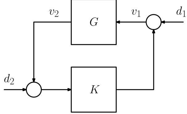
You may assume that the interconnection is well-posed (i.e. that  $I - DD_K$  is nonsingular, where  $D$  is the  $D$  matrix of the system representation  $G = (A, B, C, D)$  and  $D_K$  that of  $K = (A_K, B_K, C_K, D_K)$ ).
