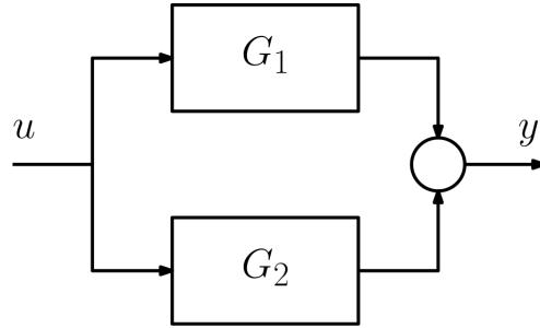
where the systems  $G_1 = (A_1, B_1, C_1, D_1)$  and  $G_2 = (A_2, B_2, C_2, D_2)$  are continuous-time, LTI systems. Assuming each signal is of a compatible dimension, derive the state and output equations of the parallel interconnection using a state vector  $x = (x_1, x_2)$  (where  $x_1$  is the state of  $G_1$  and  $x_2$  the state of  $G_2$ ), input vector  $u$ , and output vector  $y$ .
