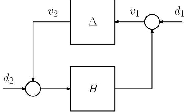
In the following, you may assume that  $H$  and  $\Delta$  have stabilizable and detectable state space realizations, and that the feedback interconnection is well-posed.
