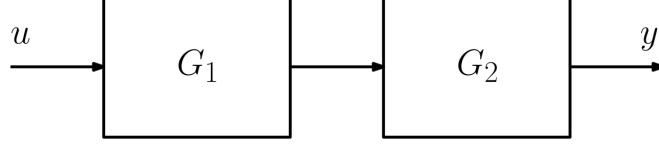
where  $G_1 = (A_1, B_1, C_1, D_1)$  and  $G_2 = (A_2, B_2, C_2, D_2)$  are continuous-time, LTI systems. Assuming each signal is of compatible dimension, derive the state and output equations of the cascade interconnection using a state vector  $x = (x_1, x_2)$ , input vector  $u$ , and output vector  $y$ .
