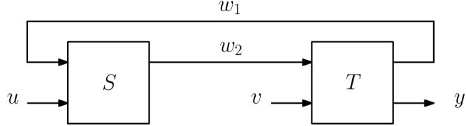
in which  $S$  and  $T$  are continuous-time, LTI systems with state and output equations,
